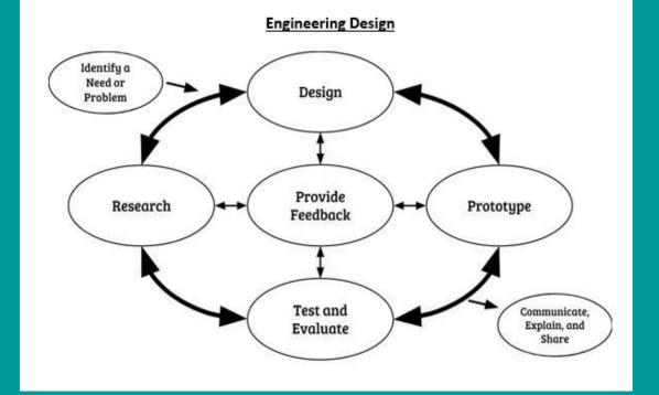
The feasibility and efficiency of the prototype must be tested and evaluated relative to the problem criteria and constraints. This includes the development of a method of testing and a system of evaluating the prototype's performance. Evaluation includes drawing on mathematical and scientific concepts, brainstorming possible solutions, testing and critiquing models, and refining the need or problem
